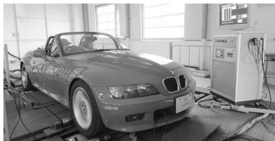
Running Test Apparatus capable of measuring speeds up to 200 kilometers per hour (BMW)
